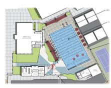
The scope of work includes replacement of two existing swimming pools with a new 25-yard x 38-meter pool for diving, swimming and water polo use, a new pool mechanical storage building, a new boys locker/shower/restroom building and associated site work, including retaining walls, concrete pool deck and walkways, and refurbishing of the existing parking lot.
